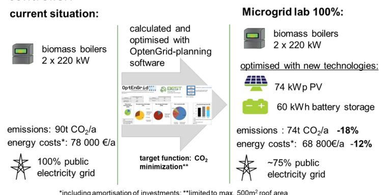
fig. 4) new technologies for cost and CO<sub>2</sub> reduction
