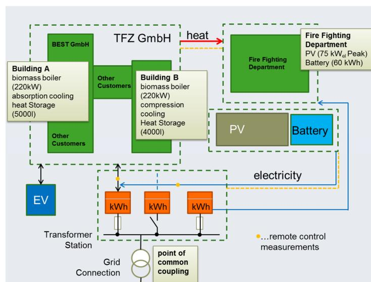
fig. 2) Concept of Microgrid Lab Wieselburg
