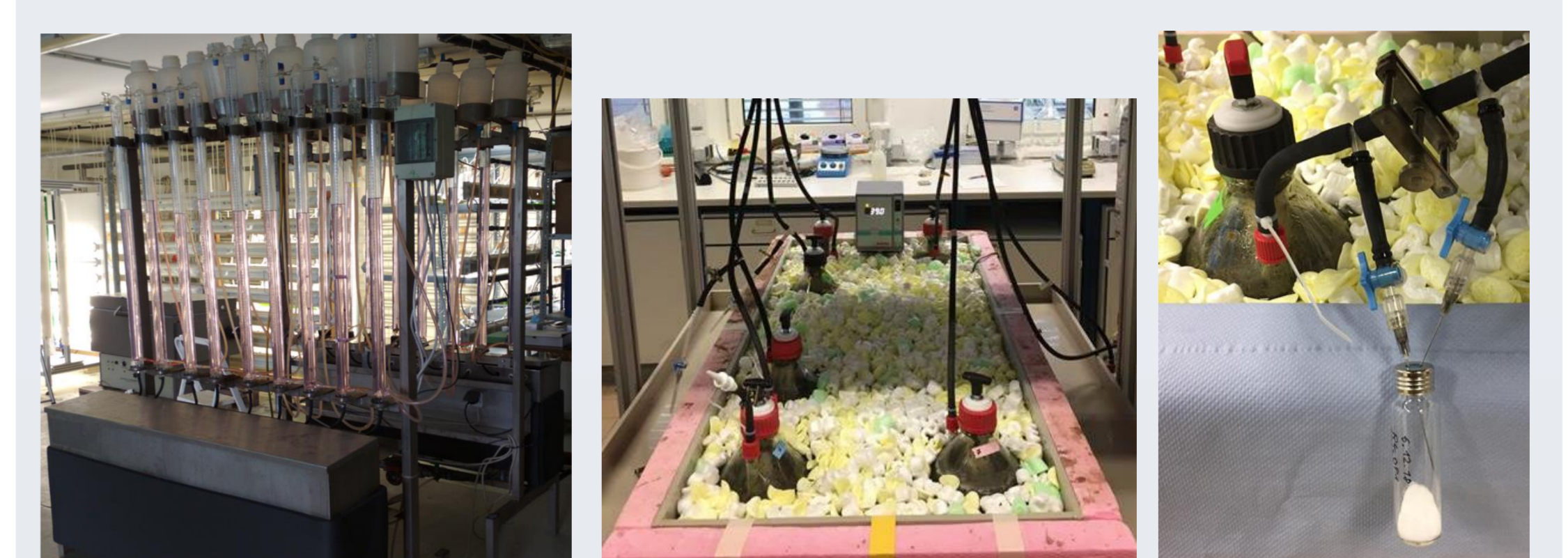
Figure 2: Eudiometer batch tests (a), semi-continuous experiments (b), terpene sampling (c)
