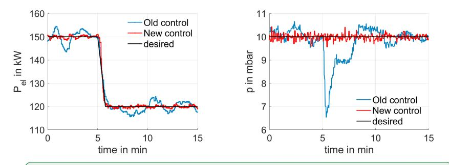
New control decreases electric power as fast but with less fluctuations
