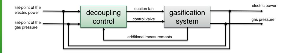
Simultaneous manipulation of the suction fan and control valve for a decoupled electric power and pressure control
