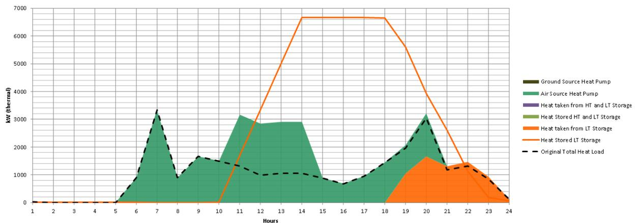
**Figure 7: Optimal Dispatch for Heating Technologies (July weekday)**
