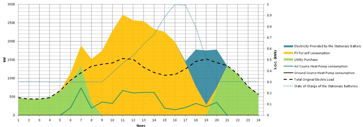
**Figure 6: Optimal Dispatch for Electricity Technologies (July weekday)**
