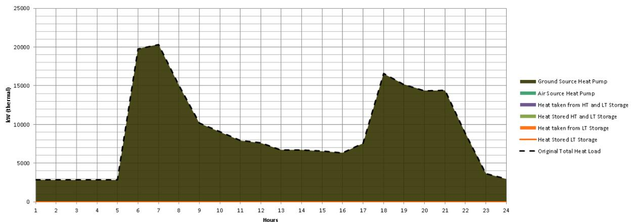
**Figure 9: Optimal Dispatch for Heating Technologies (November weekday).**
