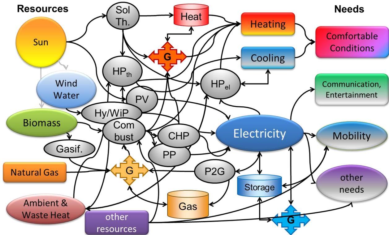
**Figure 1: Illustrating the complexity of optimizing cross-sectorial energy systems. Each of the different sectors of the energy system (here electricity, heat and gas are explicitly shown) can contain storage devices and/or grids (denoted by “G”).**
