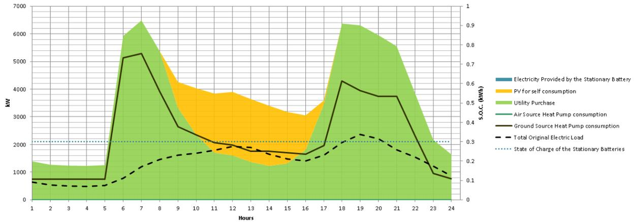
**Figure 8: Optimal Dispatch for Electricity Technologies (November weekday).**
