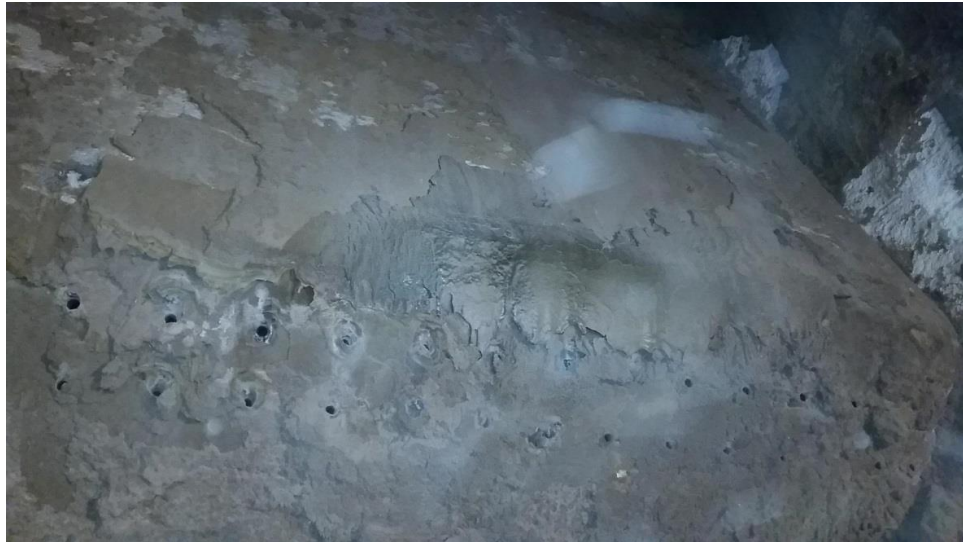
Sintered and molten ash in the furnace
