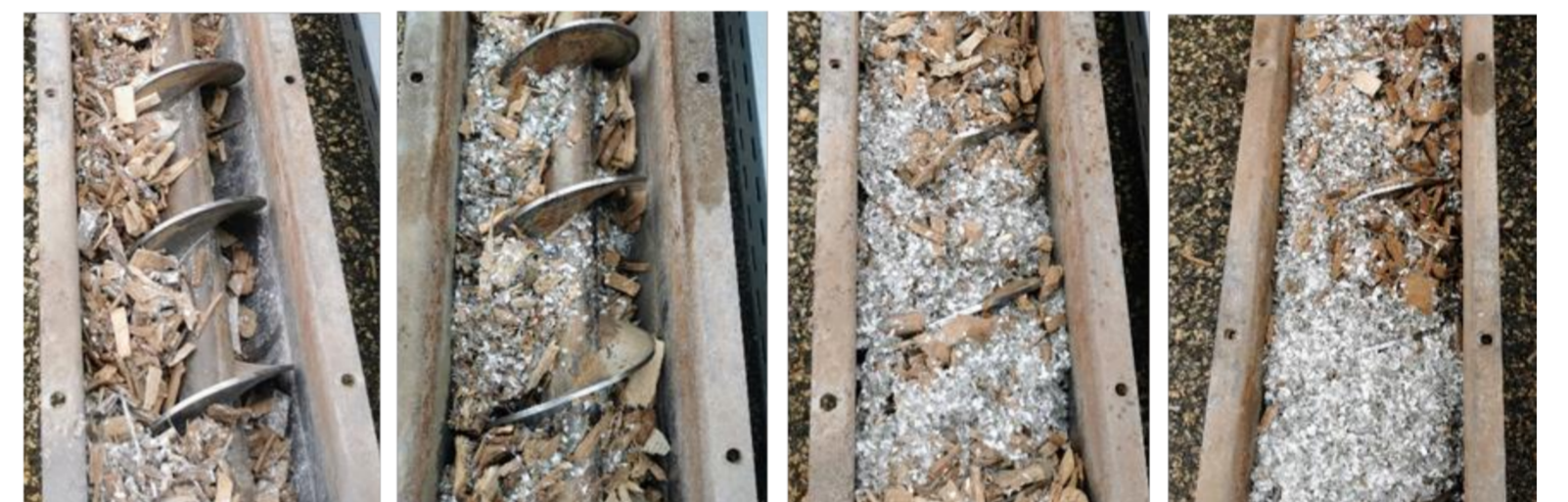
Feed conveyor after feedstock mixing, from 20% to 60% share plastics to woodchips.
