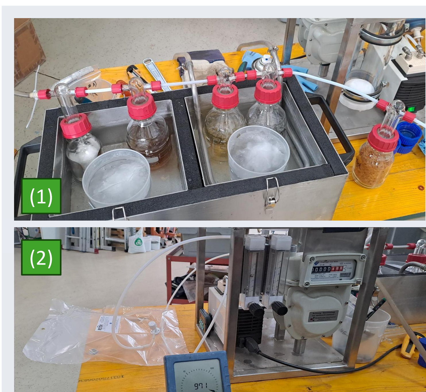
Figure 2. Gas washing with glass wool, glass frit in IPA and silicagel (1), sampling of permanent gas in tedlar bags (2)
