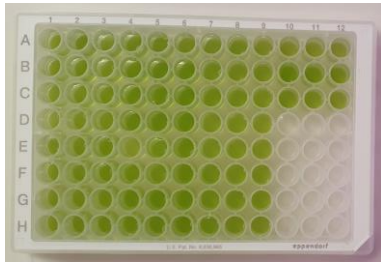
Measurement of OD_{435} , OD_{680} in 96-well plates via plate reader
